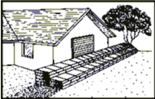
Sandbag stacking against building
